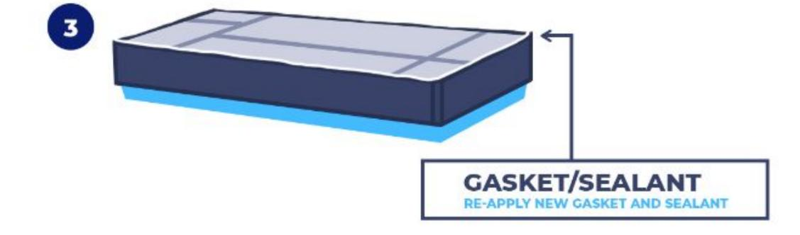
Re-Apply supplied gasket to the perimeter of the curb and around the duct drops.
