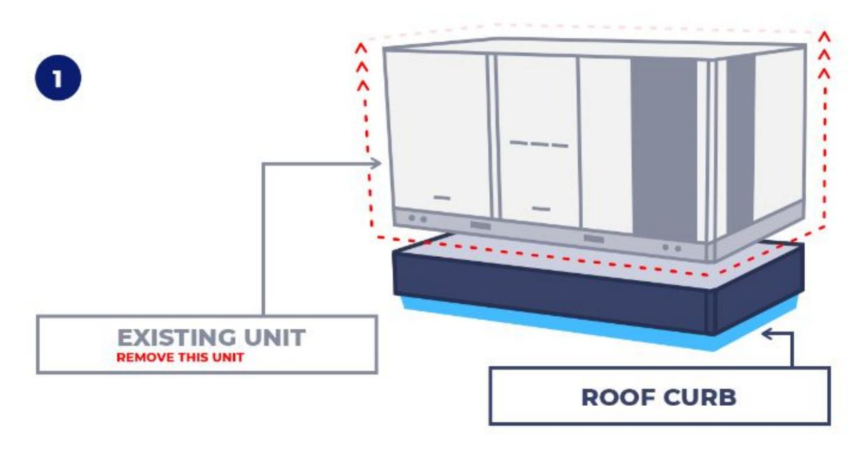
Remove the existing unit and any part of the original curb that is above the curb itself.
