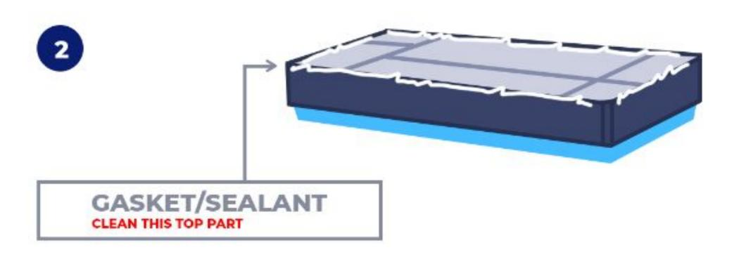
Clean the top of the existing curb rails and the duct supports removing any old gasket or sealant material.
